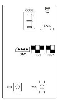
PN2: when pressed, the display shows the latest alarm code since the last time the regulator was powered. At power on, this code is "0" by default
